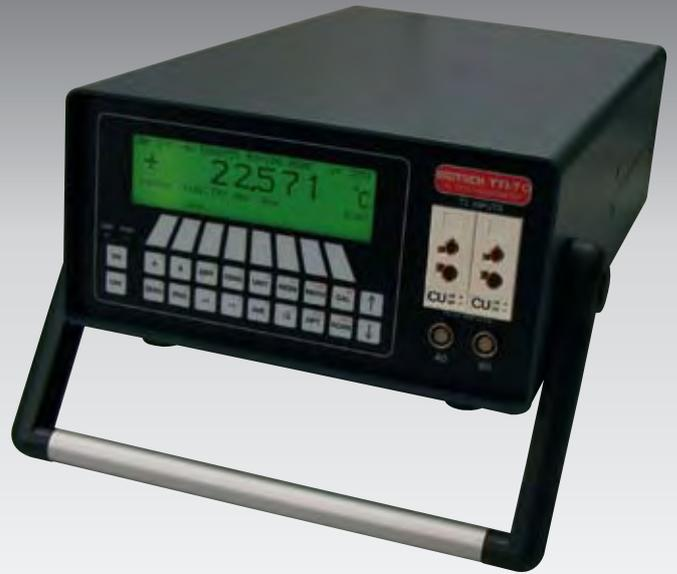
accuracy of an instrument, if you need small measurement uncertainty for high temperature PRT work you need this feature. Add the internal scanner to expand the instrument to have up to 10 channels - any or all can be scanned and lodged with the internal data logger.
