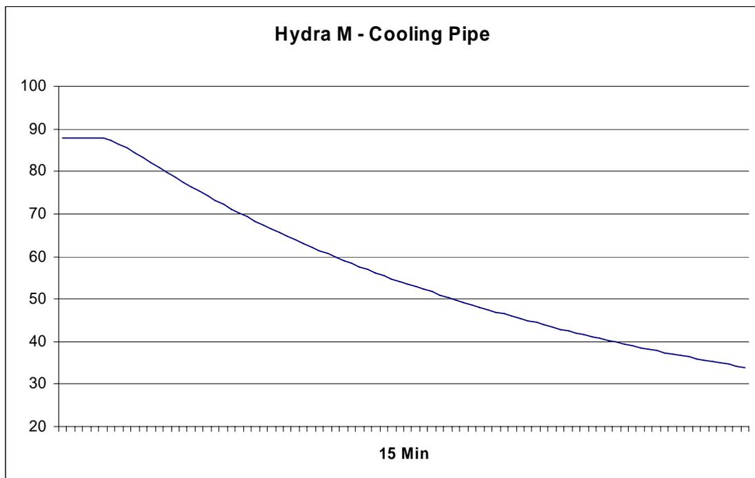
The mechanical refrigeration system runs from a nominal 40°C. The cool down time from high temperatures to the point the chiller operates is several hours. To reduce this the Hydra L and M can be used with a simple cooling pipe. Tap water can be passed through the pipe to substantially reduce the cooling time. The graph is for a Hydra M and shows the cool down time from a
